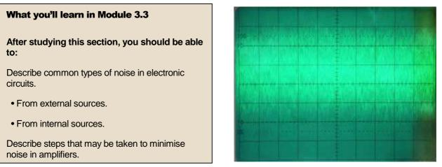
Fig. 3.3.1 CRO Displaying HF Noise
