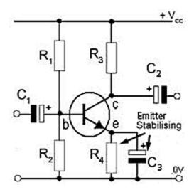
Fig 3.2.1 Emitter Stabilising Components.
