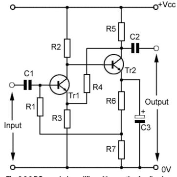
Fig. 3.2.6 DC coupled amplifier with negative feedback.
