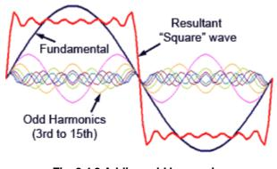
Fig. 3.4.2 Adding odd harmonics to a sine wave.
