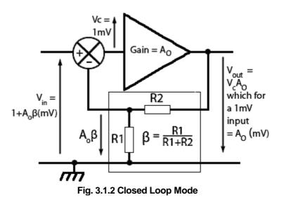
The gain of the amplifier, excluding any feedback, is  $A_o$  so that, for example, every 1mV applied across the circuit's input terminals, the amplifier will produce a phase-reversed signal of  $A_o \ge 1mV$  across the output terminals.
